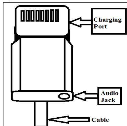
Fig. 2: Schematic of Proposed connector
