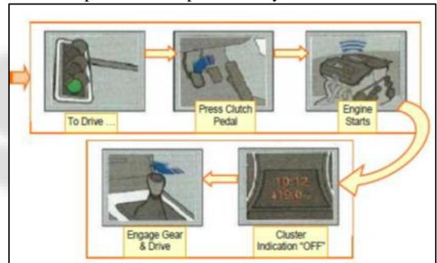
Fig. 3: Shows conditions for Auto Restart Engine
