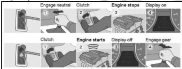
Fig. 1: Start/Stop Procedure of BMW's with Manual Transmissions
