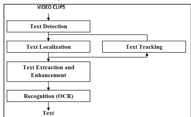
Fig. 1: Block Diagram for Extraction in Video
