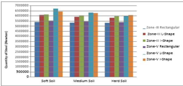
Fig. 4: quantity of steel (newton)
