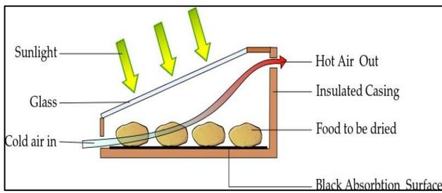
Fig. 1: Working principle of direct solar dryer
