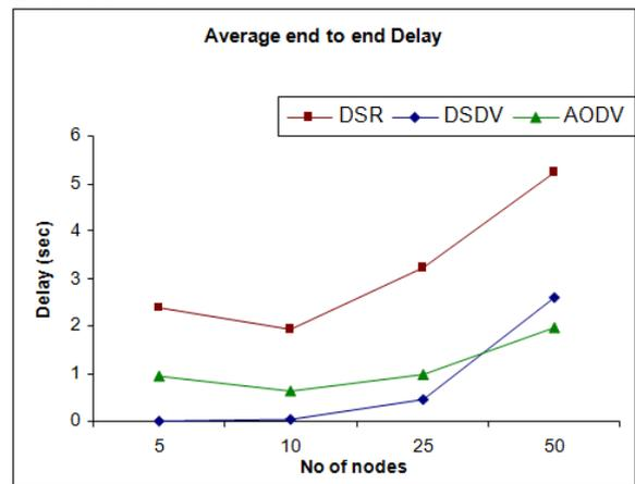
Fig. 5: Average end to end delay versus number of nodes
