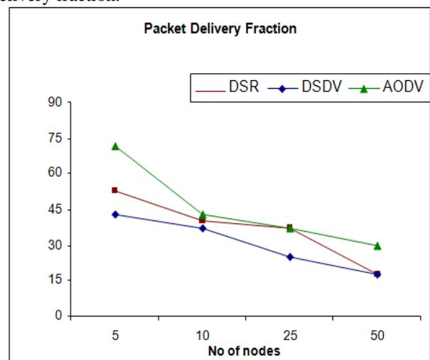
Fig. 6: Packet delivery fraction versus number of nodes
