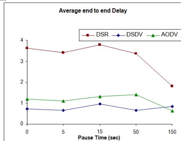
Fig. 2: Average end-to-end delay versus pause time
