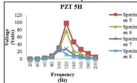
Fig. 3: Comparison of voltage generation rate of PZT 5H of different thickness by experimental method
