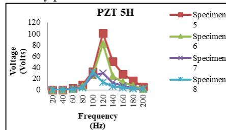
Fig. 2: Comparison of voltage generation rate of PZT 5H of different thickness by FEA method
