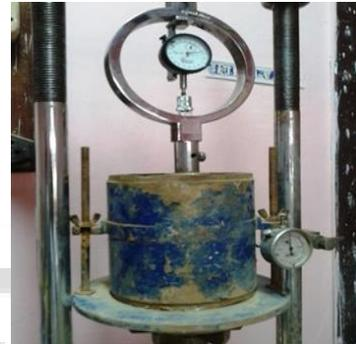
Fig. 1: CBR Apparatus
