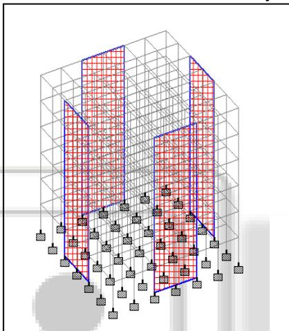
Fig. 2.4: Shear wall at middle of a 5 storey building
