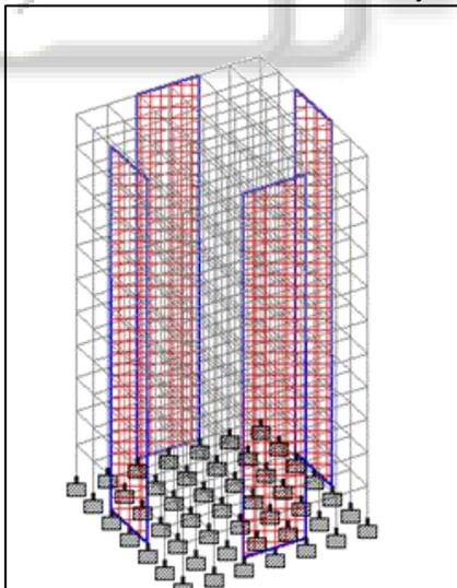
Fig. 2.5: Shear wall at middle of 10 storey building
