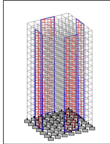
Fig. 2.6: Shear wall at middle of 15 storey building
