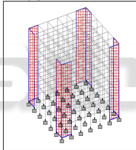
Fig. 2.1: Shear wall at corner of a 5 storey building
