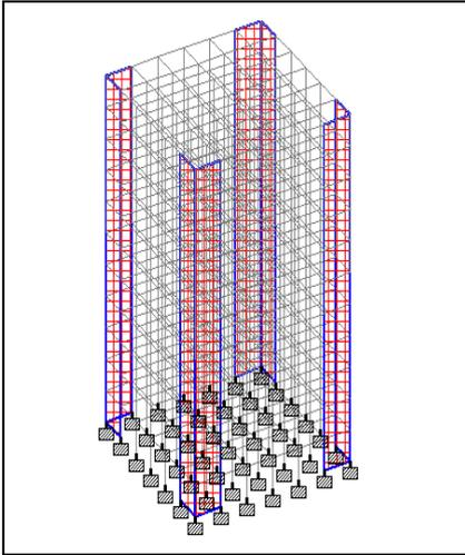
Fig. 2.3: Shear wall at corner of a 15 storey building
