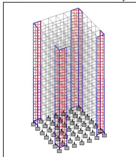
Fig. 2.2: Shear wall at corner of a 10 storey building
