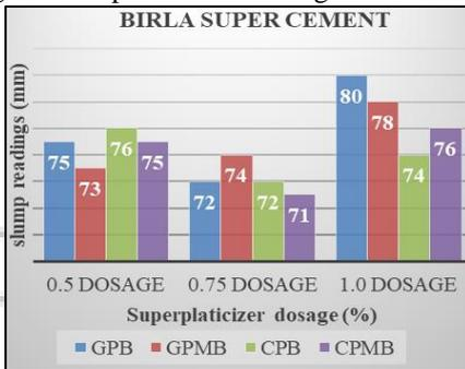
Fig. 2: Slump test results using Birla Super cement
