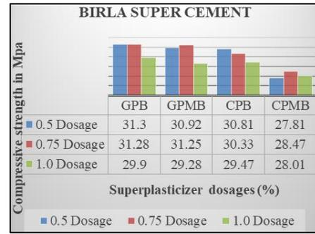
Fig. 4: Compressive strength results for 7 days using Birla super cement
