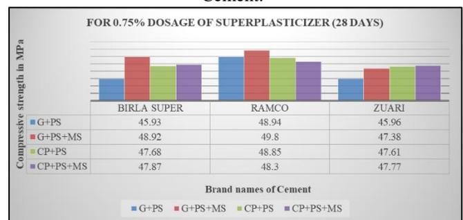
Fig. 7: Compressive strength results for 28 days at 0.75% dose of super plasticizer.
