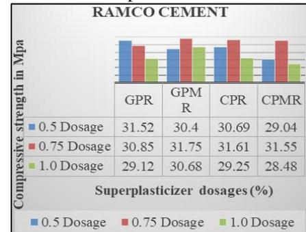
Fig. 5: Compressive strength results for 7 days using Ramco cement
