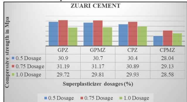
Fig. 6: Compressive strength results for 7 days using Zuari Cement.
