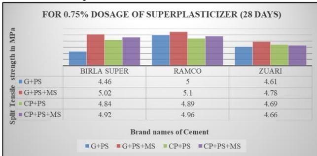
Fig. 8: Split tensile Strength results for 28days at 0.75% dose of super plasticizer
