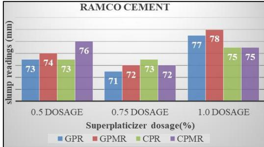
Fig. 1: Slump test results using Ramco cement
