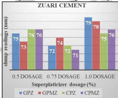
Fig. 3: Slump test results using Zuari cement
