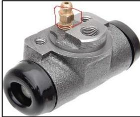
Fig. 2: Positioning of Bleeder Screw in Wheel Cylinder.
