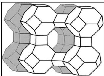
Fig. 1: Structure of Nano Hydroxy Sodalite Zeolite
