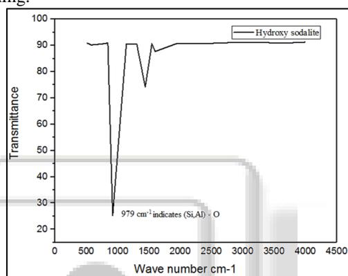
Fig. 3: FTIR spectra of Nano Hydroxy Sodalite zeolite
