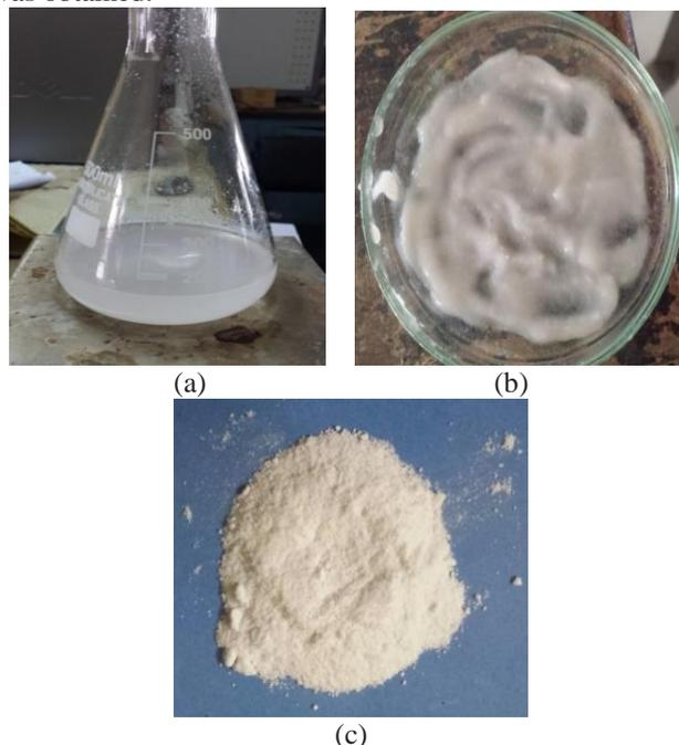
Fig. 2: a) Mixed solution of sodium aluminate and sodium silicate. (b) nano hydroxy sodalite zeolite in wet condition. (c) Fine powder of nano hydroxy sodalite zeolite.
