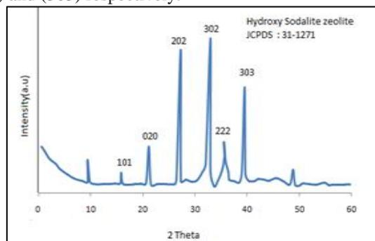
Fig. 4: XRD pattern of Nano Hydroxy Sodalite zeolite
