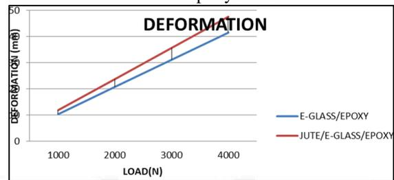
Fig. 6: Load Vs Deformation
