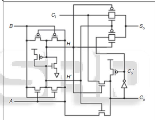
Fig. 1: Circuit schematic of LPHS-FA[13]
