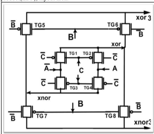
Fig. 2: Three input and 16T XOR/XNOR using transmission gate(XO4)[20]
