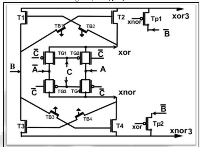
Fig. 4: Three input and 18T XOR/XNOR using transmission gate (XO10)[20]
