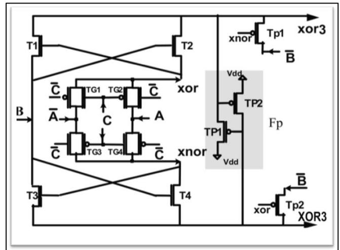
Fig. 3: Three input and 16T XOR/XNOR using transmission gate (XO7)[20]
