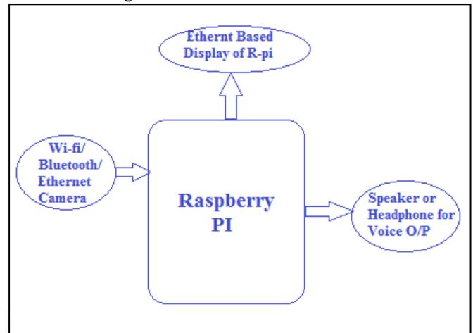
Fig. 1: Raspberry Pi Based OCR System Block Diagram
