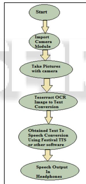
Fig. 4: Process Flow Block Diagram
