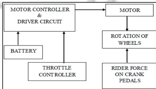
Fig. 1: Components of Electric Bicycles [2]
