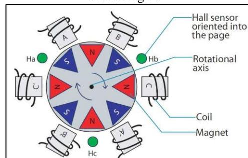
Fig. 3: Permanent magnet BLDC construction [2]
