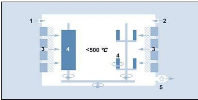
Fig. 2.1: Schematic Diagram of PVD process
