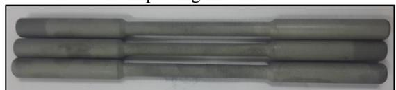
Fig. 3.3: Sand Blasted Specimens
