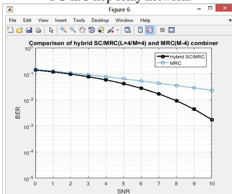
Fig. 7: Comparison between hybrid combiner and MRC
