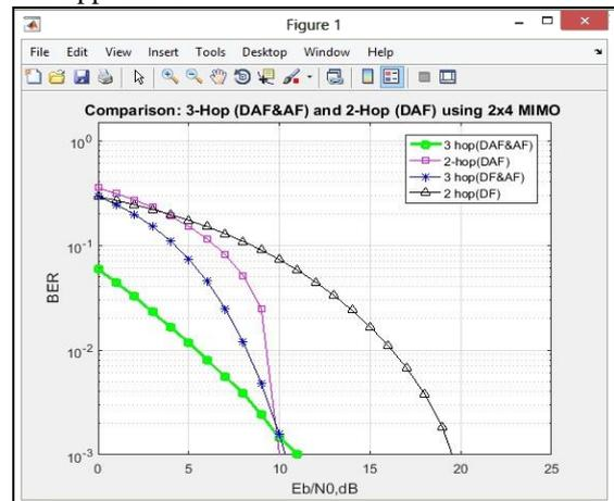
Fig. 3: Comparison of 3 hop (DAF&AF), 3 hop (DF and AF) in 2X4 MIMO
