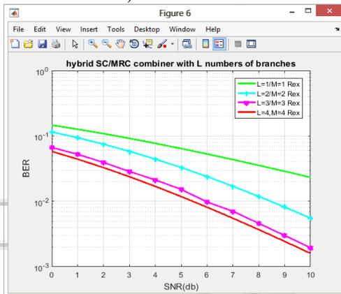
Fig. 5: Hybrid SC/MRC combiner with different L/M branches
