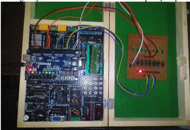
Fig. 10: Implementation on FPGA(Spartan 3E)
