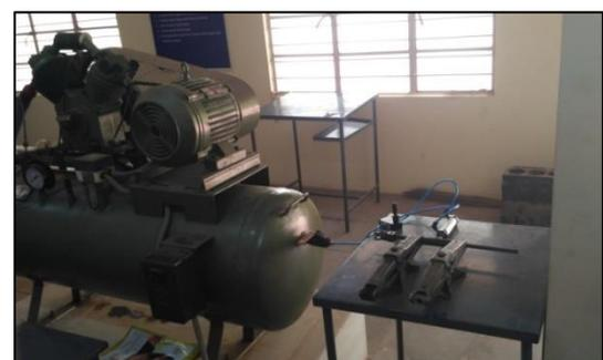
Fig. 8: Pneumatic Operated Bed lifter
