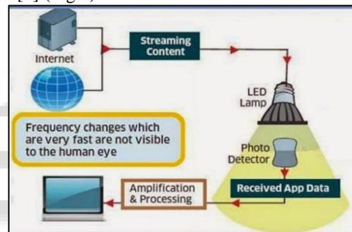
Fig. 2: Block diagram of Li-Fi Sub System
