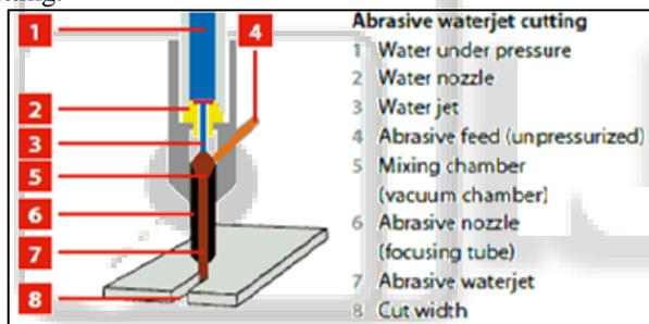
Fig. 8: Abrasive jet machine
