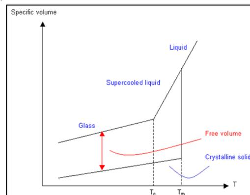
Fig. 1: Phase transformation of crystalline and amorphous solids on heating.
