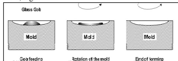
Fig. 6: Spinning Process
