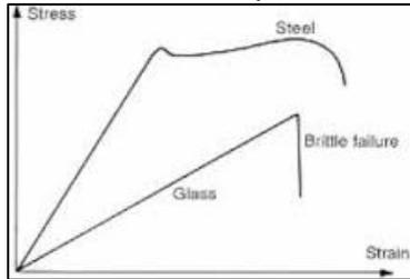
Fig. 2: stress strain curve of glass and steel
