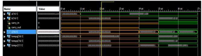
Fig. 9: Simulation result of adder design
