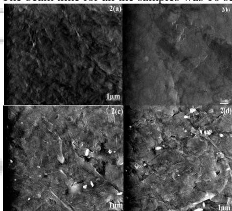
Fig. 2: FE-SEM images of ion-beam treated pristine and grafted PTFE (a) Pristine (b) Grafted at temperature 50°C (c) Grafted at temperature 60°C (d) Grafted at temperature 70°C. The beam time for all the samples was 100 seconds
