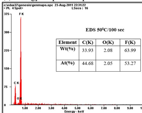
Fig. 3(b): Energy Dispersive Spectrum of treated PTFE (Beam Time=100 sec) with grafting temperature 50°C
