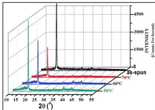
Fig. 5: Comparative analysis of XRD images of pristine with treated PTFE grafted at 50°C, 60°C and 70°C temperature
