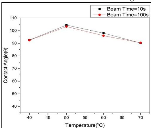
Fig. 4: Variation of contact angle with grafted temperature of PTFE with beam time of 10 sec and 100 sec.
