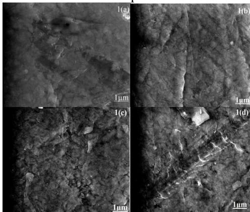
Fig. 1: FE-SEM images of ion-beam treated pristine and grafted PTFE. (a) Pristine (b) Grafted at temperature 50°C (c) Grafted at temperature 60°C (d) Grafted at temperature 70°C. The beam time for all the samples was 10 seconds.
