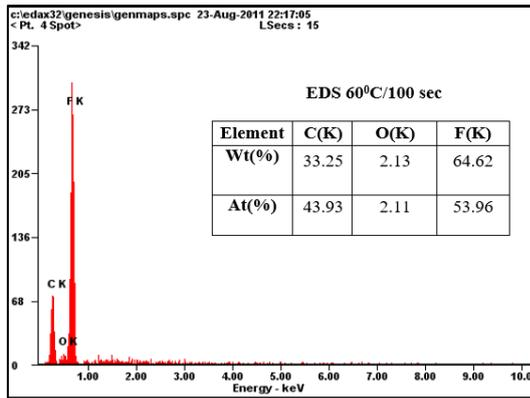
Fig. 3(c): Energy Dispersive Spectrum of treated PTFE (Beam Time=100 sec) with grafting temperature 60°C
