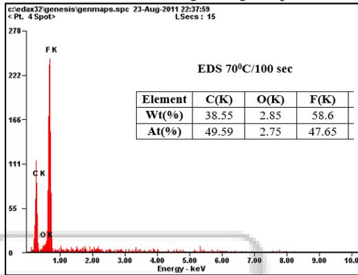
Fig. 3(d): Energy Dispersive Spectrum of treated PTFE (Beam Time=100 sec) with grafting temperature 70°C
