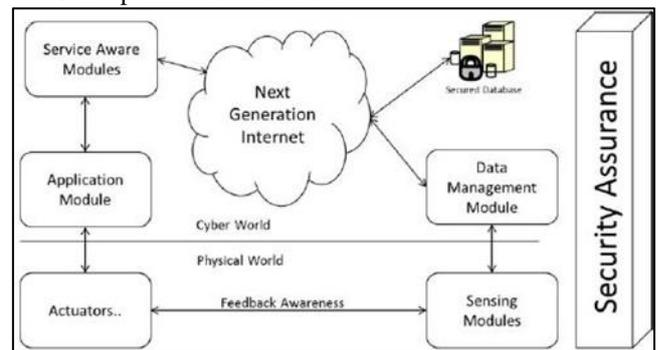
Fig. 4: CPS Design - Modules & Components
