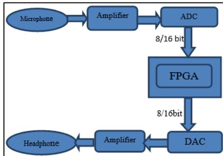
Fig. 1: Block diagram for the audio de-noising
