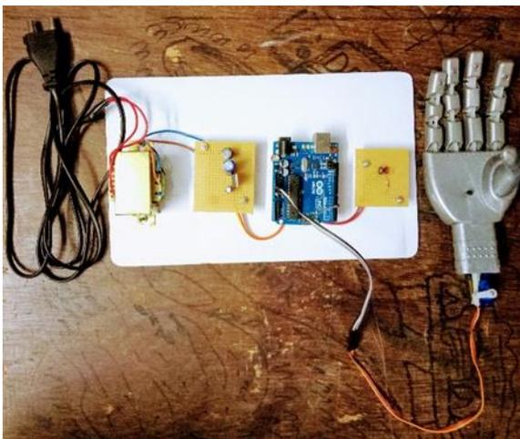
Fig. 3: Sensor based robotic wrist for adaptive grasping. If any object is given to our designed product, it can automatically adapt for the same by the use of axis sensor and force sensors. (See Fig. 3)
