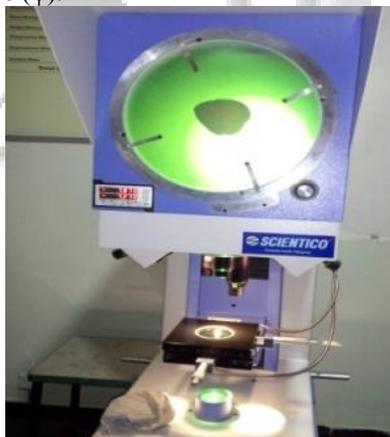
Fig. 5: Size measurement of sample pearls (profile projector)
