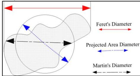
Fig. 2: Schematic of different particle diameters in 2D image
