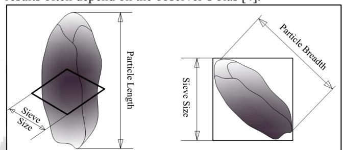
Fig. 1: Particle passing through a sieve aperture
