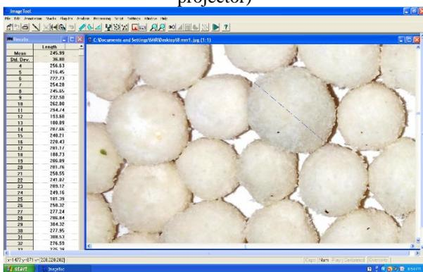
Fig. 6: Measurement of particle size using the UTHSCSA ImageTool 3.0
