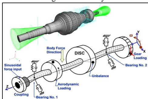
Fig. 1.1: Basic Diagram of Rotor Dynamics
