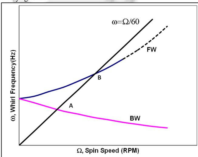
Fig. 1.3: Analytical Campbell Diagram for a Simple Rotor
