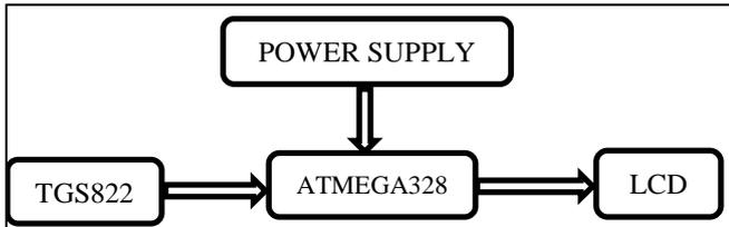
Fig. 1. Block Diagram of the Hardware.
