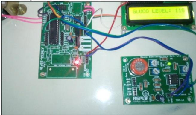
Fig. 4: Experimental Setup for glucose measurement
