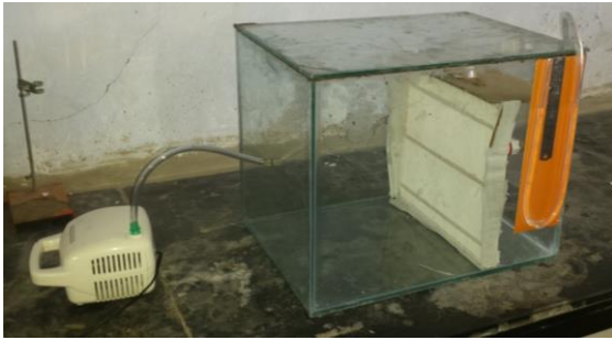
Fig. 5: Testing of HEPA filter at MHSSCOE
