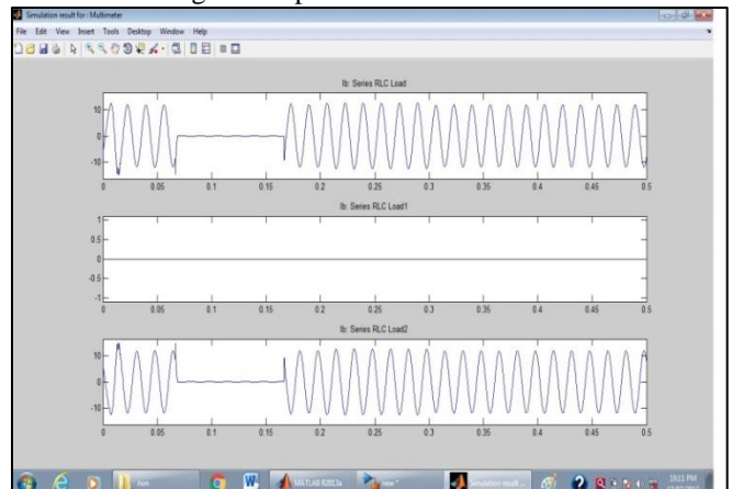
Fig. 10: RLC Load MultiMeter Voltage and Current
