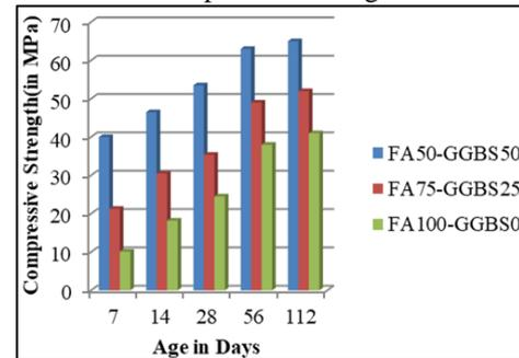
Fig. 1: Compressive strength versus Age
