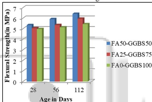
Fig. 3: Flexural strength of mixes
