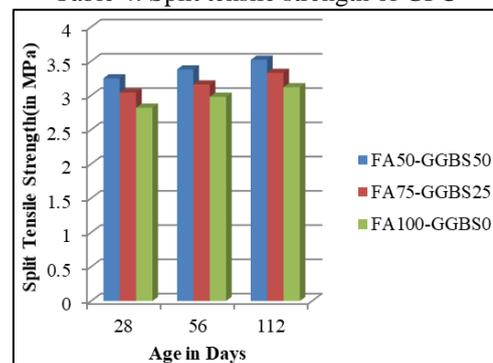
Fig. 2: Split tensile strength of mixes
