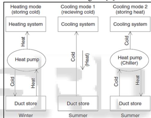
Fig. 4: Operational principles for ATEs systems using heat pumps [6]
