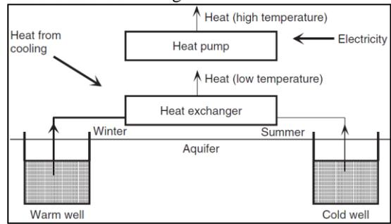
Fig. 3: A schematic of ATEs system combined with a heat pump [6]
