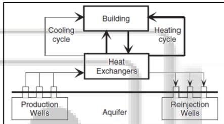
Fig. 1: Schematic of Aquifer thermal energy storage [6]
