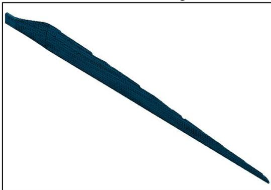
Fig. 3: Monolithic Wind Turbine blade mesh
