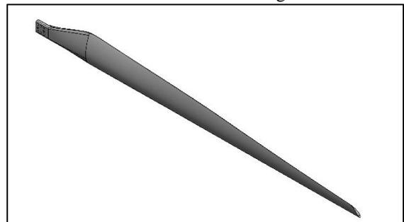
Fig. 1: Isometric view of Monolithic Wind Turbine Blade
