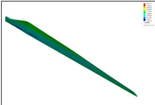
Fig. 4: Surface Pressure Distribution
