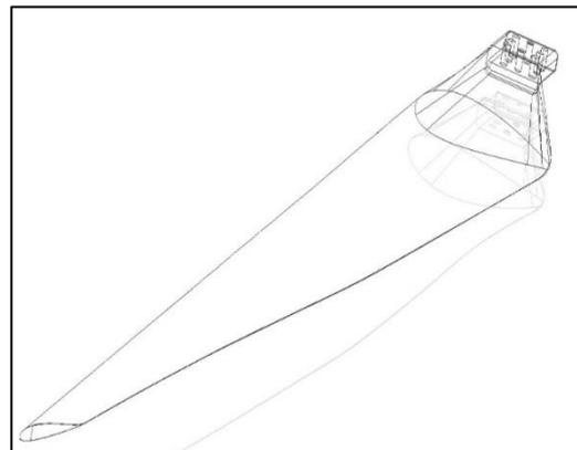
Fig. 2: Wireframe model of Monolithic Wind Turbine Blade
