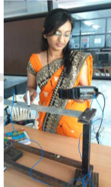
Fig. 5: Experimentation with the cantilever beam.
