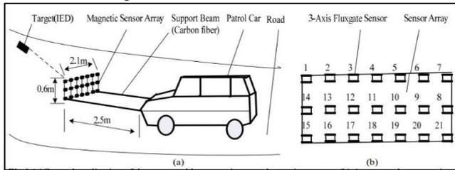
Fig. 2: (a) General application of the car-portable magnetic anomaly sensing system. (b) Are tangularma genetic sensor array of twenty-one 3-axis fluxgate sensors.
