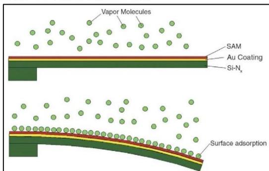
Fig. 3: Diagram showing molecular-adsorption-induced bending of a cantilever arising from differential adsorption. The adsorption decreases the free energy, which changes the surface stress.
