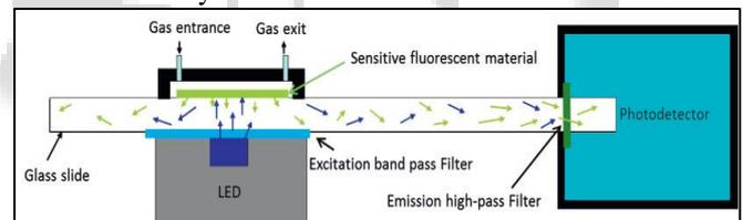
Fig. 1(a): Concept of the fluorescent detector device;
