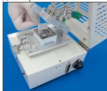
Fig. 1(b): DESORB device
