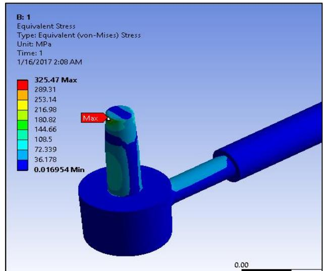
Fig. 5.2: Equivalent stress for filleting the edge by 1 mm radius
