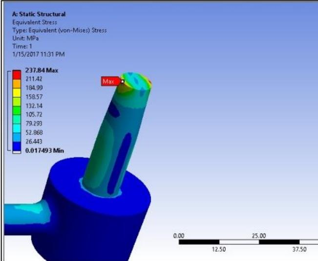
Fig. 5.1: Maximum equivalent stress (von-mises)
