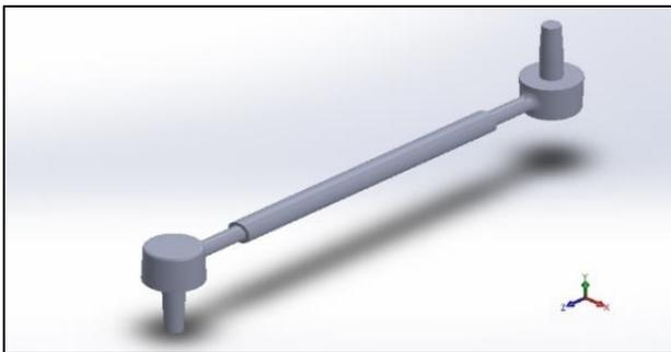
Fig. 3.1: The original 3D model of TIE ROD
