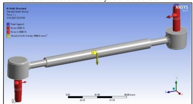
Fig. 4.2: boundary conditions and forces acting on the tie rod
