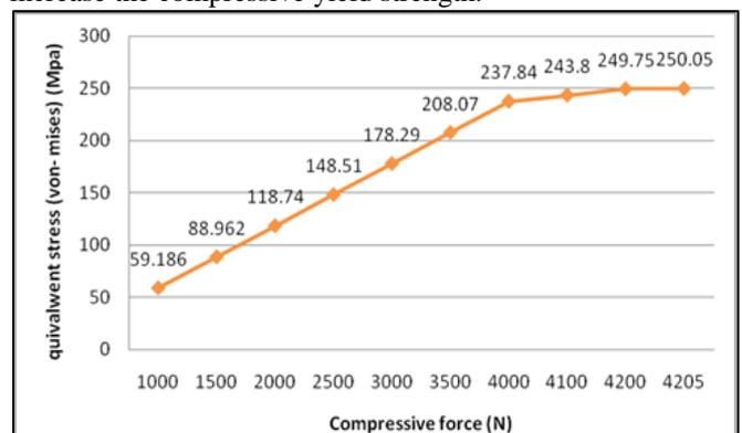
Graph 4.1: compressive force vs. Equivalent stress (von-mises)
