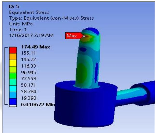
Fig. 5.3: Equivalent stress for filleting the edge by 5 mm radius
