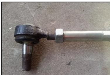
Fig. 1.1: A vehicle tie rod
