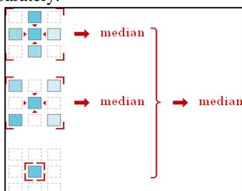
Fig. 3: Hybrid Median filter operation
