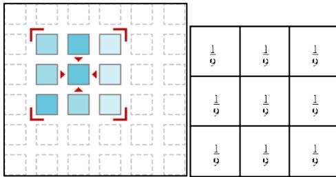
Fig. 2: 3 x 3 kernel used for mean filter
