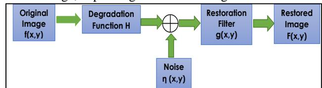
Fig. 1: Image degradation and restoration model
