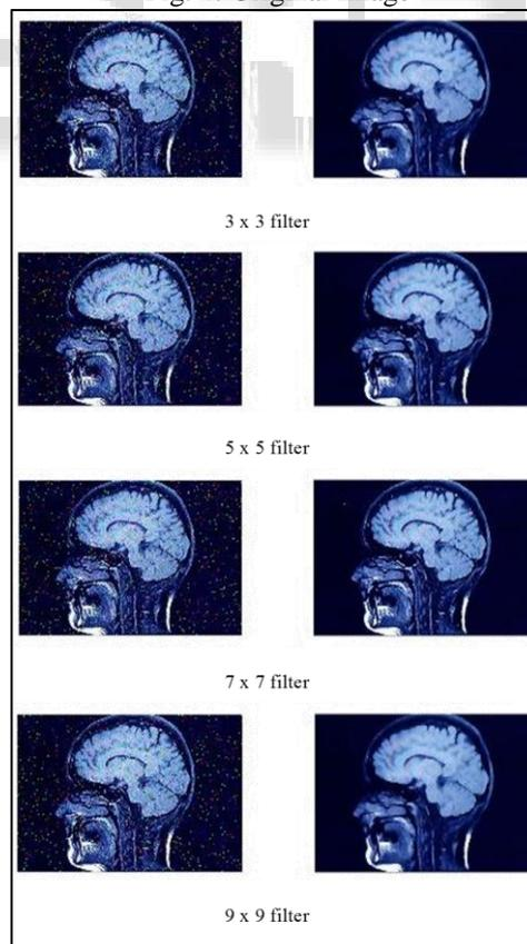
Fig. 5: Hybrid Median Filters for salt and pepper noise removal (3%noise)
