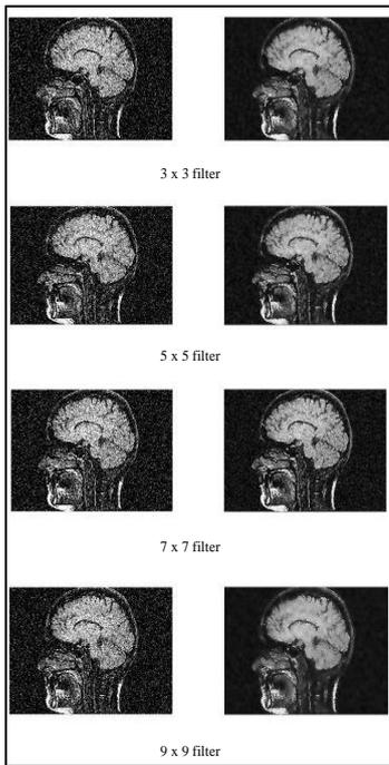
Fig. 6: Adaptive Wiener Filters for Gaussian noise removal (3% noise)
