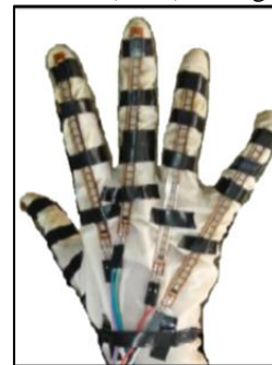
Fig. 1: Flex Sensors mounted on the Hand glove
