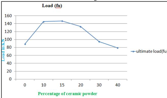
Fig. 14: Graphical representation of above flexural strength results
