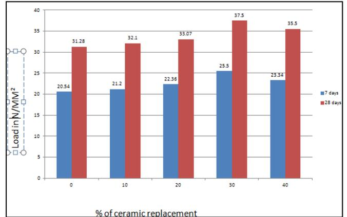
Fig. 11: Compressive strength results in graphical representation
