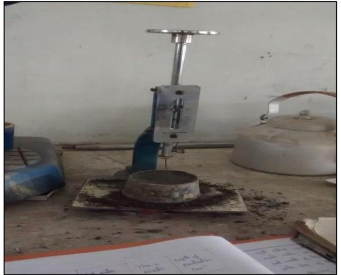
Fig. 8: Initial setting time test
