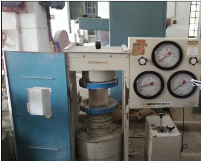
Fig. 9: Compressive Strength testing machine
