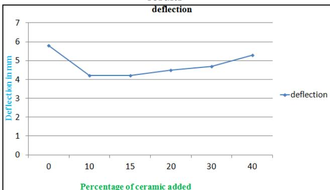
Fig. 15: Graphical representation of deflections from above results
