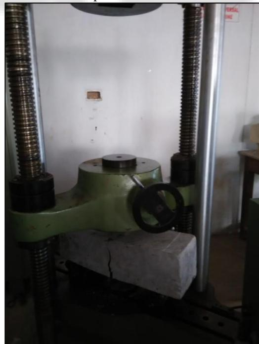
Fig. 12: UTM Machine for Flexural Strength testing
