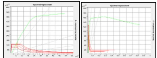
Fig. 11: Performance point as per 440 FEMA Equivalent Linearization Full Infill wall (Push X and Push Y)
