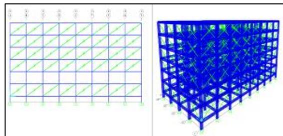
Fig. 5: Elevation & 3D View of G+5 soft storey at first floor.
