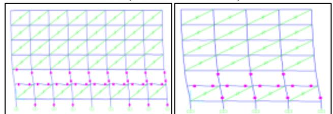
Fig. 16: Deformed shape and plastic hinge formation for performance point Soft Storey at First Floor (Push X and Push Y)
