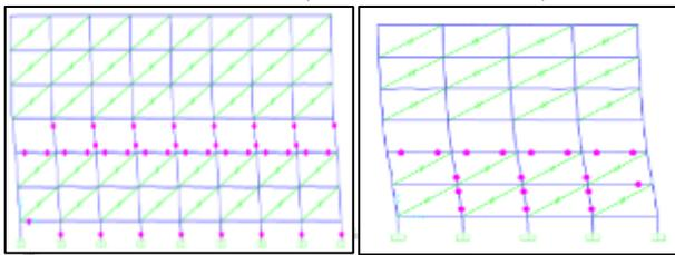
Fig. 19: Deformed shape and plastic hinge formation for performance point Soft Storey at Second Floor (Push X and Push Y)
