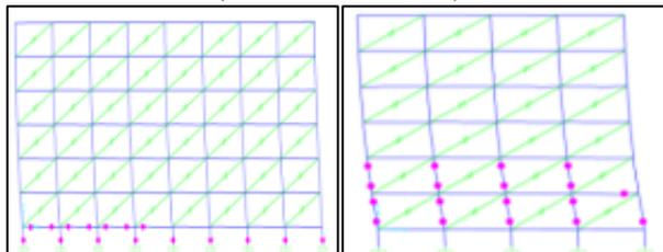
Fig. 10: Deformed shape and plastic hinge formation for performance point Full Infill wall (Push X and Push Y)
