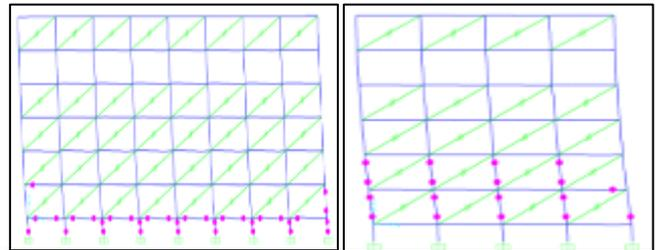
Fig. 25: Deformed shape and plastic hinge formation for performance point Soft Storey at Fourth Floor (Push X and Push Y)
