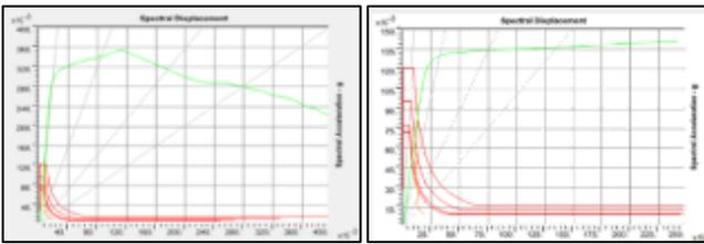
Fig. 17: Performance point as per 440 FEMA Equivalent Linearization Soft Storey at First Floor (Push X and Push Y)
