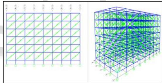
Fig. 3: Elevation & 3D View of G+5 storey infill wall frame building
