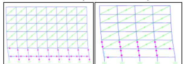
Fig. 13: Deformed shape and plastic hinge formation for performance point Soft Storey at Ground Floor (Push X and Push Y)
