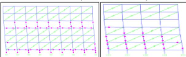
Fig. 22: Deformed shape and plastic hinge formation for performance point Soft Storey at Third Floor (Push X and Push Y)
