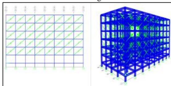
Fig. 4: Elevation & 3D View of G+5 soft storey at ground floor.
