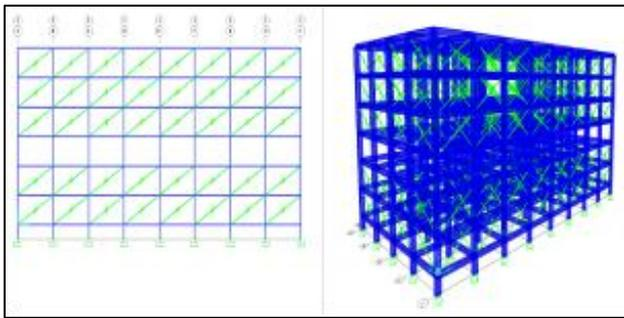
Fig. 6: Elevation & 3D View of G+5 soft storey at second floor.
