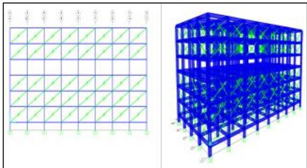
Fig. 7: Elevation & 3D View of G+5 soft storey at third floor.
