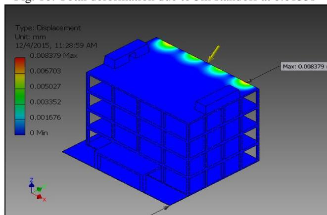
Fig. 11: Total deformation due to 5m standoff at 0.015s
