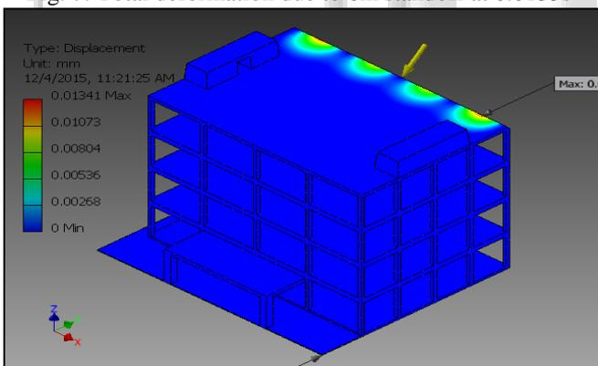
Fig. 8: Total deformation due to 6m standoff at 0.015s
