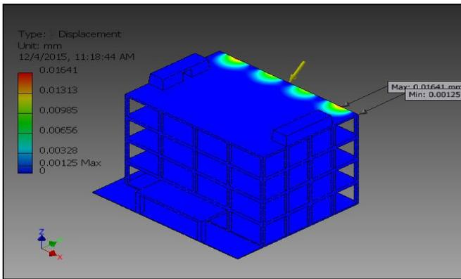
Fig. 6: Total deformation due to 6m standoff at 0.0094s
