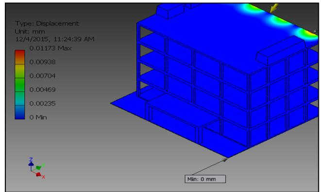
Fig. 10: Total deformation due to 5m standoff at 0.0135s
