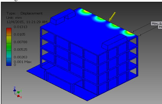
Fig. 9: Total deformation due to 5m standoff at 0.0094s
