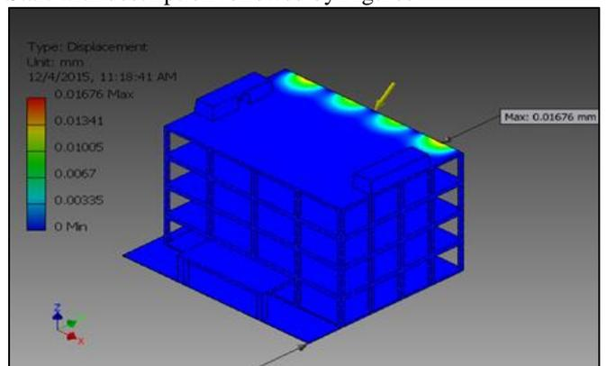
Fig. 5: Total deformation due to dead load and live load alone
