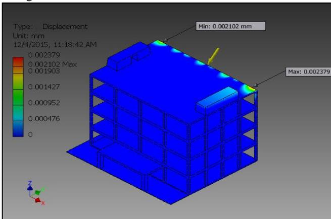
Fig. 7: Total deformation due to 6m standoff at 0.0135s
