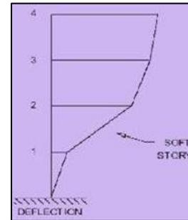
Fig. 3: Soft story behavior of a building structure under lateral loading
