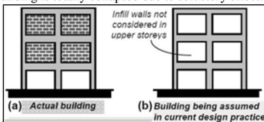
Fig. 5: Assumptions made in current design practice are not consistent with the actual structure
