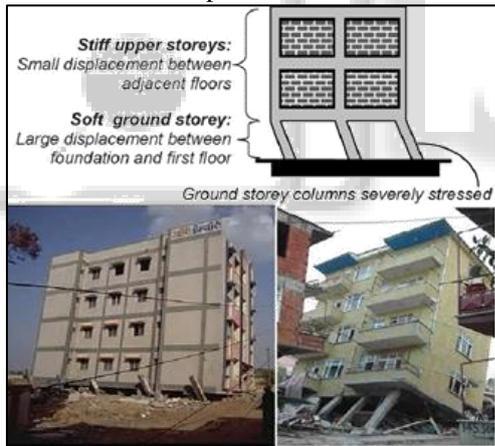
Fig. 2: Failure due to large lateral displacement in soft story
