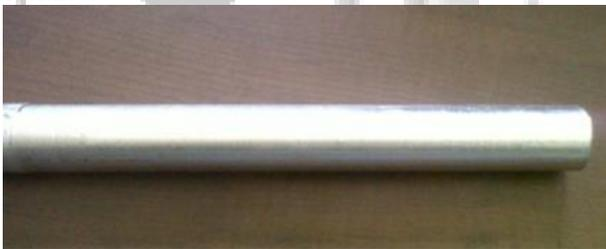
Fig. 10: Test Specimen A356
