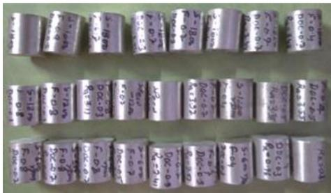
Fig. 11: Side view of specimen for roughness measurement after turning
