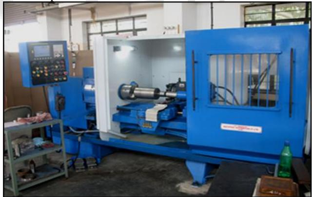
Fig. 7: Experimental setup (CNC lathe)
