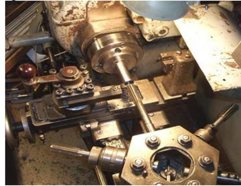
Fig. 3: Turret lathe
