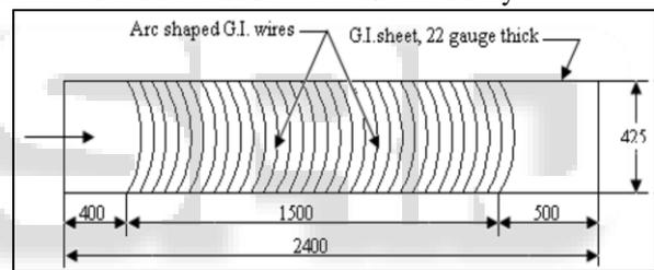
Fig. 1: Arc shaped roughness on Absorber plate investigated by Saini and Saini
