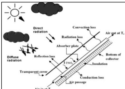
Fig. 1: Solar air heater constructional details
