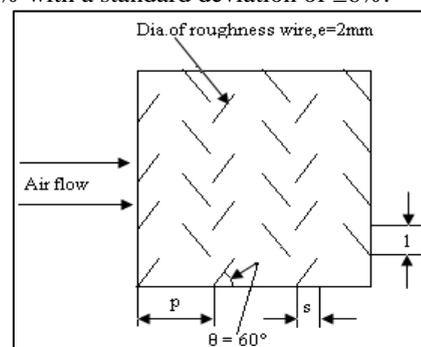
Fig. 2: Layout of roughness surface investigated by Karmare and Tikekar
