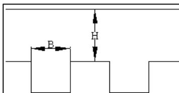
Fig. 4: Grid arrangement for grooved channel flow investigated by Eiamsa-ard and Promvonge
