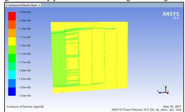
Fig. 12: Density plot for vertical heating coil arrangement.
