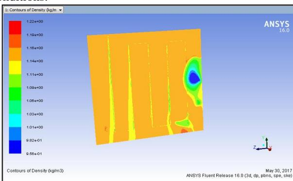
Fig. 10: Density plot for horizontal heating coil arrangement
