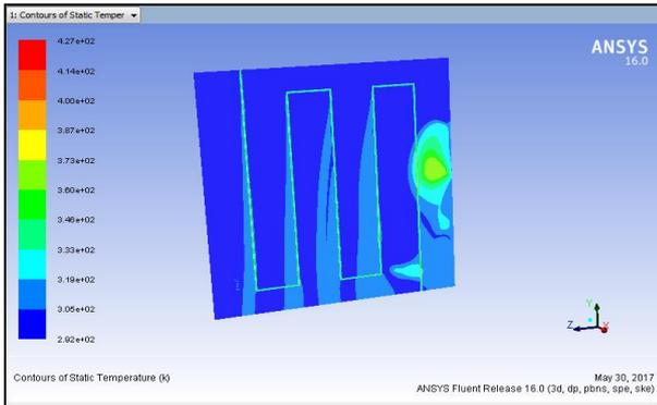
Fig. 9: Temp plot for horizontal heating coil arrangement
