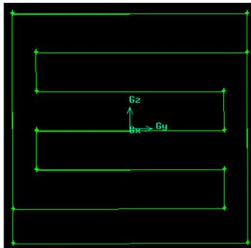
Fig. 4: Heating coil horizontal arrangement in Gambit interface
