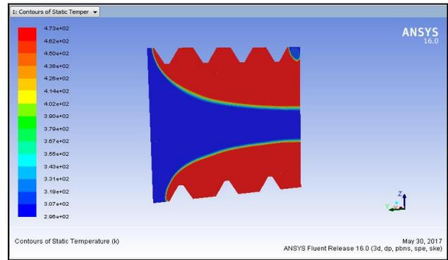
Fig. 13: Temp plot for nozzle inserts configuration
