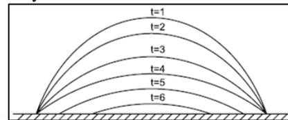
Fig. 2: Droplet shape evolution during evaporation
