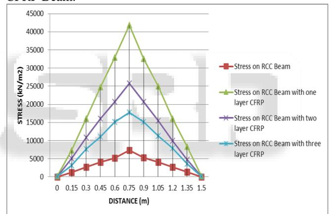
Fig. 5: Effect of Stress on RCC Beam
