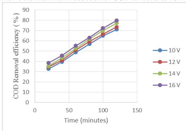
Fig. 4: Effect of Voltage on COD
