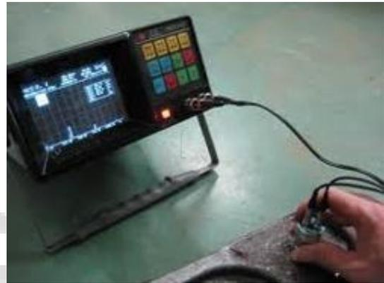
Fig. 3: Ultrasonic testing arrangement
